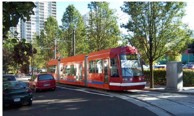
Figures 3 and 4 – At left is an example of a visually unobtrusive single contact wire (ETB) streetcar system in Portland, OR. The photo at right is of Essex Street in Jersey City, where the Hudson Bergen Light Rail line runs in two directions. It is a single wire OCS (cross cabling is support wire to reduce sagging). It also shows the dedicated Light Rail Vehicle lane at left; the right lane is mixed use traffic.
