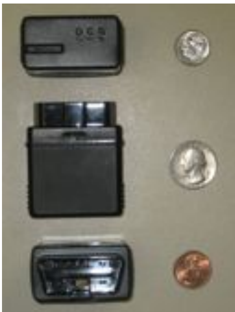
OBD vehicle tracking device, consisting of a GPS receiver, cellular transceiver, and microprocessor. Image by author.
