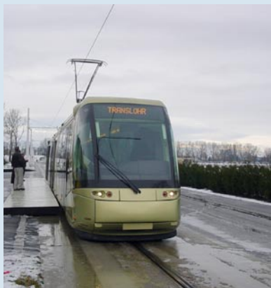
Translohr rubber tire test vehicle, which is bi-directional, at the Lohr Industries test track in Obernai, France. System utilizes traditional catenary and traction power design and is planned or in service in Italy and France. Vehicles are modular units and are designed to operate completely in a fixed-guideway.
